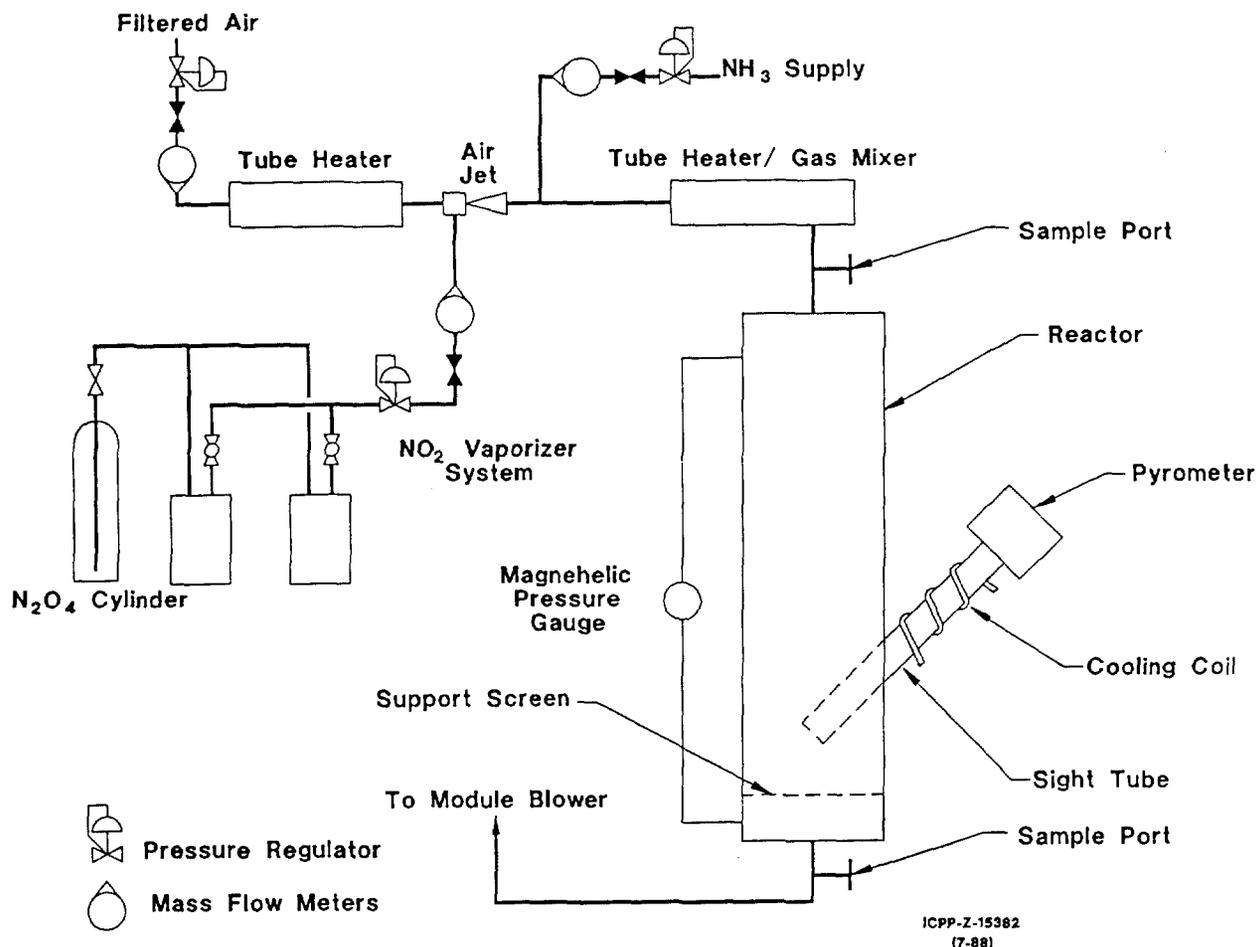
Figure 1. Simplified  $\text{NO}_x$  abatement laboratory-scale reactor system schematic.
