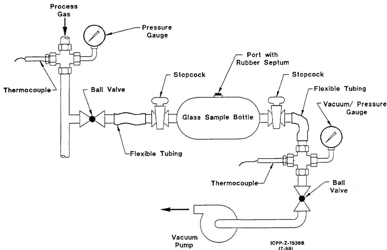
Figure 5. Schematic of vacuum extraction sampling system.
