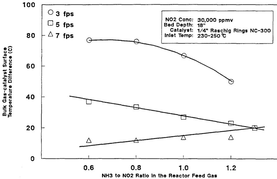
Face Velocity and NH<sub>3</sub> /NO<sub>2</sub> Effects on the Bulk Gas to Catalyst Surface Temperature Difference
