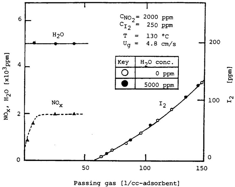
Fig.6 Effect of the presence of NO<sub>x</sub> on the breakthrough curve of iodine.
