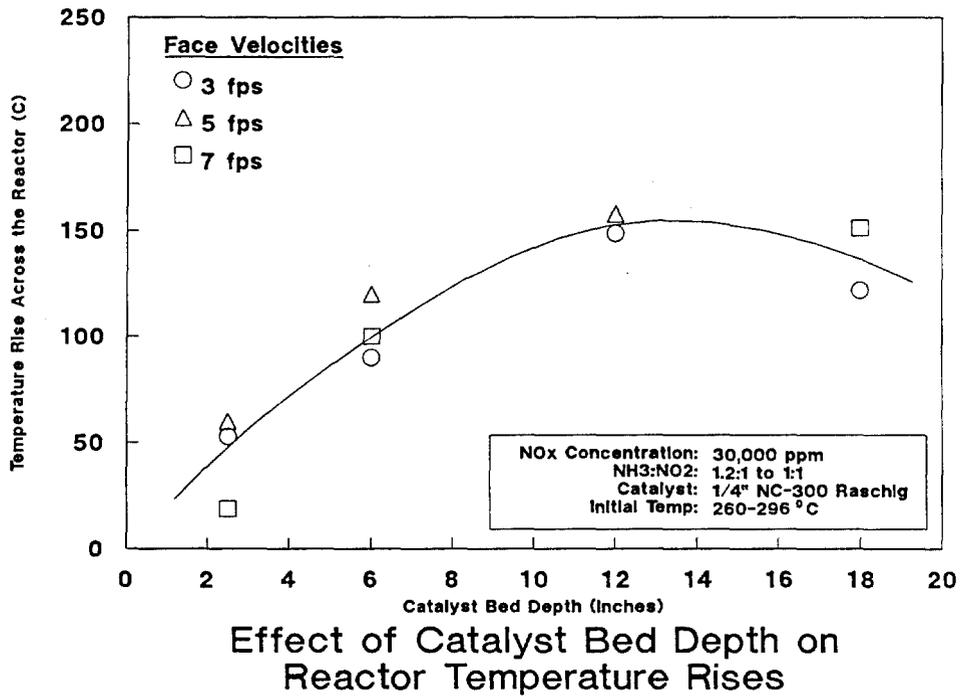
Effect of Catalyst Bed Depth on Reactor Temperature Rises
