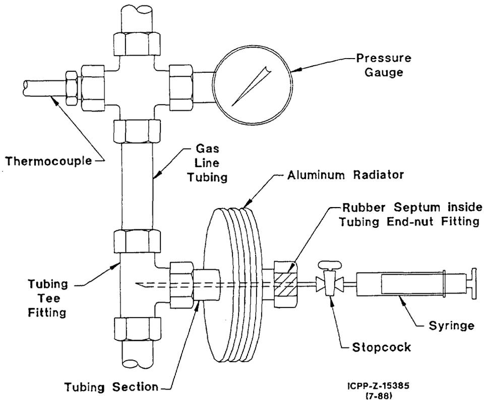
Figure 4. Schematic of syringe extraction sampling system.
