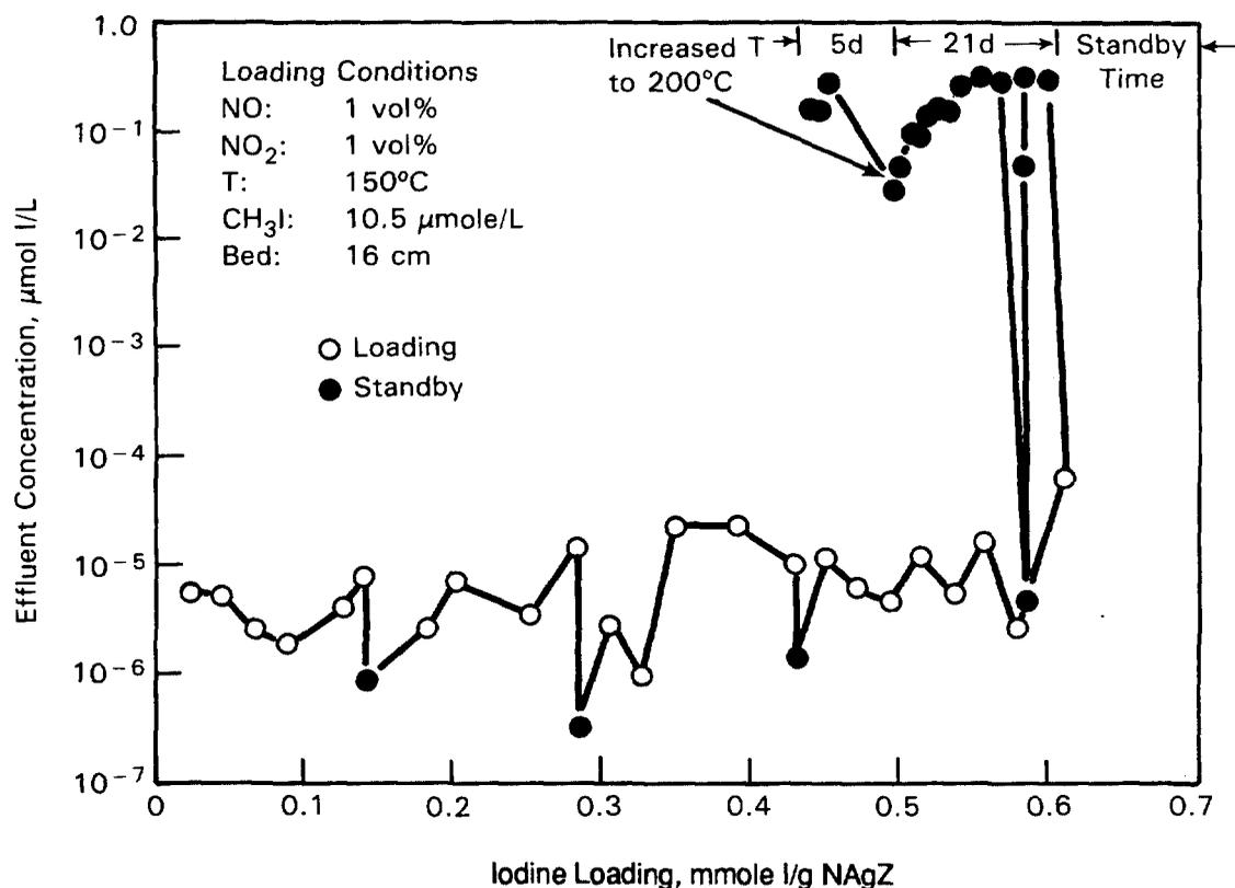
FIGURE 3. Effluent Concentration vs Iodine Loading on NAgZ for the Extended Standby Test
