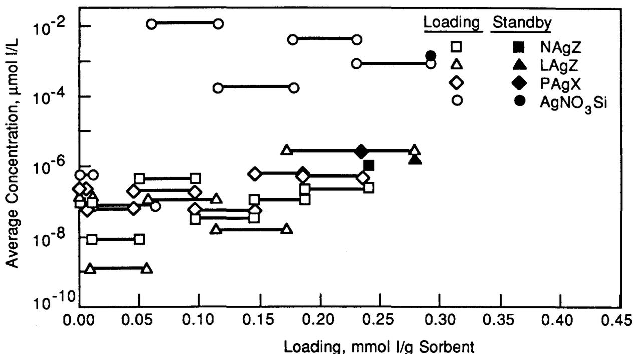
FIGURE 4. Average Effluent Concentrations from Beds of NAgZ, LAgZ, AgX, AgNO<sub>3</sub>Si (Shutdown/Startup Cycles performed at nominal loadings of 0.01, 0.05, and 0.15 mmol I/g Sorbent)
