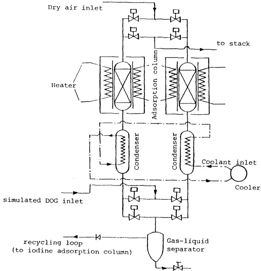
Fig.8 Schematic diagram of thermal swing adsorption process.
