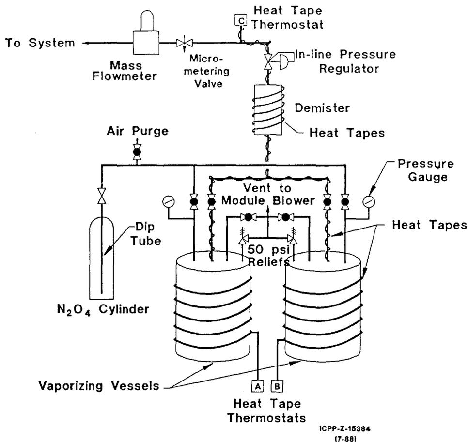
Figure 3. Schematic of NO<sub>2</sub> vaporizer system.
