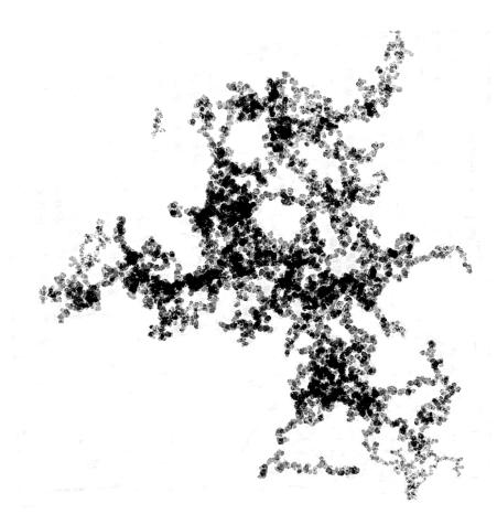
The lower density deposits may account for the increased plugging by carbon black compared to test dust.
