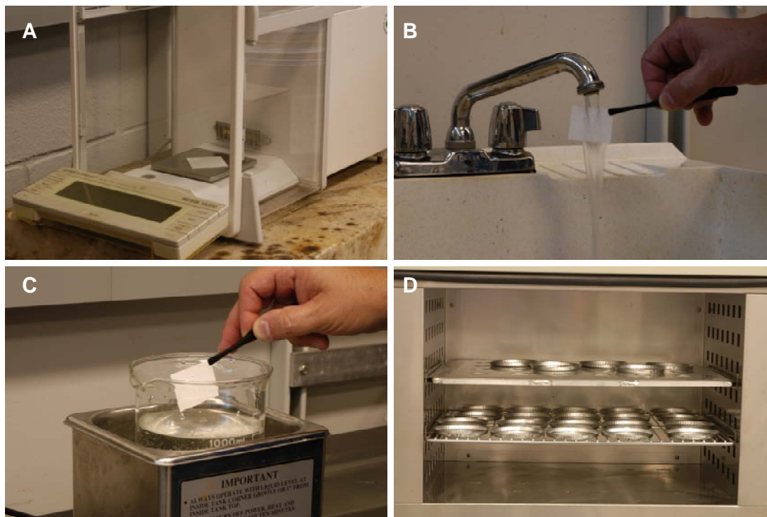
Figure 11. A: Weighing 5x5 grid sections. B: Washing 5x5 grid sections under flowing tap. C: Sonicating 5x5 grid sections. D: Drying 5x5 grid sections.
