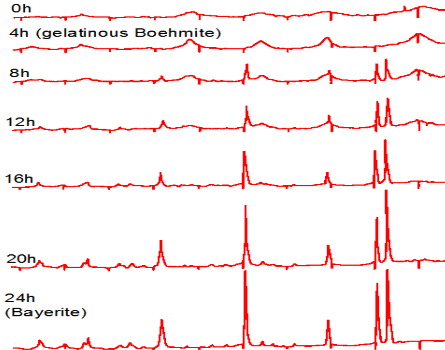
Aging of Aluminum Hydroxide Gel, pH 9, 300K, X-Ray Patterns (Wefers & Misra)
