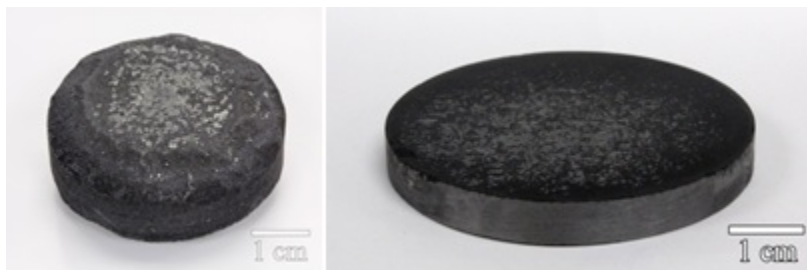
Figure 1: Pucks of iodine-loaded Ag 0 -aerogel produced with HIP (left) and SPS (right) (Matyáš et al. 2015)
