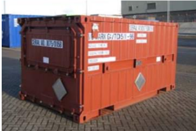
Figure 6 – Low level waste storage container [8]
