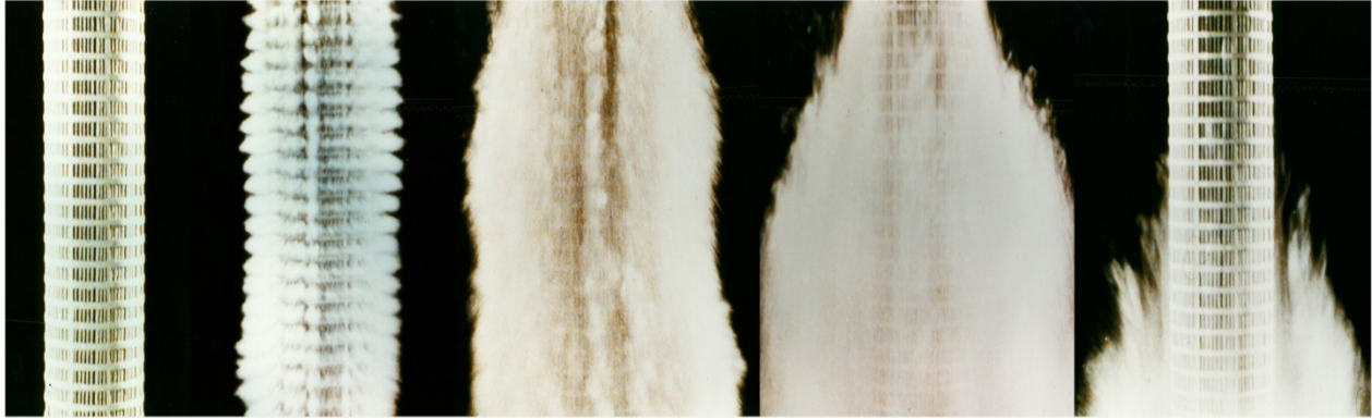
Fig. 4 Pulse Jet cleaning of Metal Media HEPA Filter
